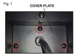
A. Remove the cover plate from the right side bottom of the appliance by removing the three screws, as shown above. Save screws for Installation of new cover plate.
